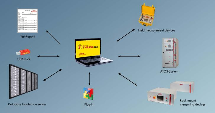
The T-Base software package is a powerful tool for remote control, data exchange, result analysis and sequence for a completely automated test. It runs on every Windows based PC. A modern graphical user interface makes it easy and comfortable to operate. Any additional features can easily be created with a custom Plug-In.
